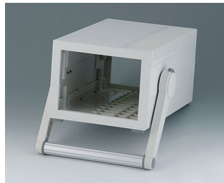
B2212307 MEDITEC E 220, with handle bar ABS (UL 94 HB) off-white RAL 9002 160x260x124mm IP 40
