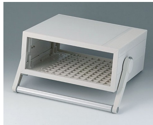
B2210307 MEDITEC D 220, with handle bar ABS (UL 94 HB) off-white RAL 9002 290x260x124mm IP 40
