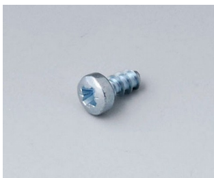
A0306031 Self-tapping screws 3 x 6 mm (PZ1)
