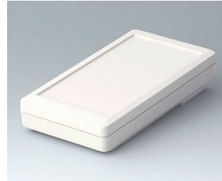
A9073117 DATEC-MOBIL-BOX S, Vers. I ABS (UL 94 HB) off-white RAL 9002 152x83x33,5mm IP 65 opt.
