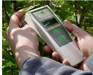
Chlorophyll fluorimeter for plant screening
