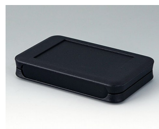
A9051209 SOFT-CASE M PMMA (IR) (UL 94 HB) black RAL 9005 65x105x19mm IP 54 opt., IP 40
