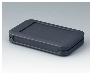
A9050108 SOFT-CASE S ABS (UL 94 HB) lava 51x82x14mm IP 54 opt., IP 40
