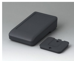
A9005218 DATEC-COMPACT S ASA+PC (UL 94 V-0) lava 136x74x32mm IP 41
