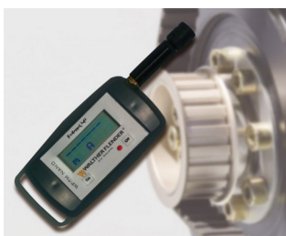
Tension meter for measuring belt pretension
