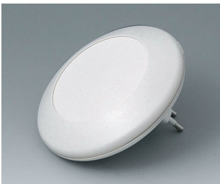
B5011227 ART-CASE R110 F PC+ABS (UL 94 V-0) off-white RAL 9002 ø110x38mm IP 40
