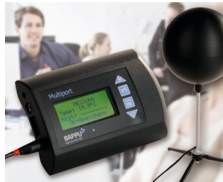
Multiport with integrated datalogger
