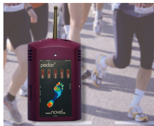
Dynamic pressure measuring between foot and shoe
