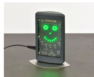
Room air measuring device
