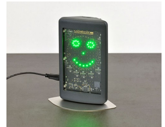
Room air measuring device
