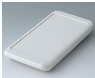
B5403307 SLIM-CASE M, Vers. III ASA+PC (UL 94 V-0) off-white RAL 9002 148x74x19mm IP 65 opt., IP 40
