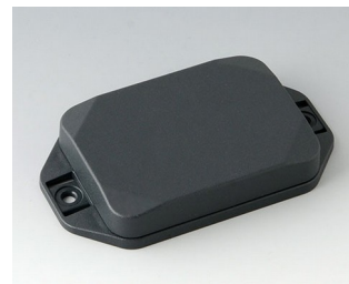
B1824128 MINI-DATA-BOX EF50, flat, with flanges ASA+PC (UL 94 V-0) anthracite grey RAL 7016 70x50x15mm IP 65 opt., IP 40
