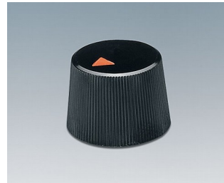
A1316240 TUNING KNOB, with lateral screw fixing ABS (UL 94 HB) black RAL 9005 16,4x12,3mm 4mm
