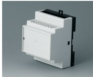
B6503115 RAILTEC B, 4 modules, Vers. II PC (UL 94 V-0) light grey RAL 7035 70x86x58mm
