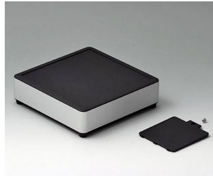
ES143059 SYNERGY S140 Aluminium AIMgSi 0,5 matt anodised 140x140x40mm IP 40
