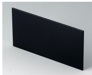
B6143222 Rear panel PPO (UL 94 V-0) black RAL 9005 119,1x62,7x2,2mm
