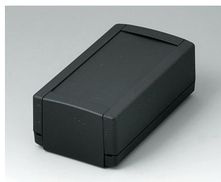
B1050369 TOPTEC 123 H, Vers. I ABS (UL 94 HB) black RAL 9005 123x68x45mm IP 40
