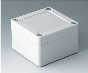
C7008011 IN-BOX ABS (UL 94 HB) gris clair RAL 7035 84x82x55mm IP 66, IP 67, IK 07
