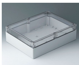
C7030105 IN-BOX PC gris clair RAL 7035 302x232x90mm IP 66, IP 67, IK 08
