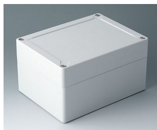
C7016062 IN-BOX PC gris clair RAL 7035 162x122x90mm IP 66, IP 67, IK 08
