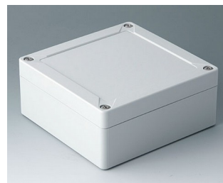
C7013031 IN-BOX ABS (UL 94 HB) gris clair RAL 7035 124x122x55mm IP 66, IP 67, IK 07
