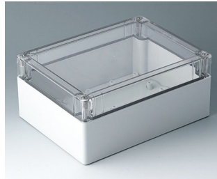
C7021074 IN-BOX ABS/PC (UL 94 HB) gris clair RAL 7035 202x152x90mm IP 66, IP 67, IK 07
