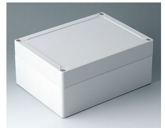
C7021071 IN-BOX ABS (UL 94 HB) gris clair RAL 7035 202x152x90mm IP 66, IP 67, IK 07
