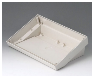
B4026117 DATEC-TERMINAL SL ABS (UL 94 HB) gris blanc RAL 9002 264x180x86mm IP 54 opt.
