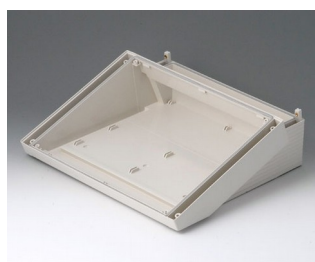
B4030117 DATEC-TERMINAL L, Vers. I ABS (UL 94 HB) gris blanc RAL 9002 302x272x101mm IP 54 opt.
