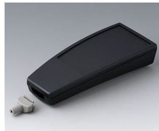
A9068139 SMART-CASE XL, Vers. IV ABS (UL 94 HB) noir RAL 9005 168x74,4x35,4mm IP 65 opt., IP 40
