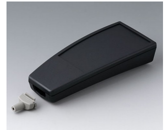
A9068139 SMART-CASE XL, Vers. IV ABS (UL 94 HB) noir RAL 9005 168x74,4x35,4mm IP 65 opt., IP 40
