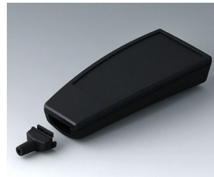
A9067339 SMART-CASE L, Vers. IV ABS (UL 94 HB) noir RAL 9005 140x62,7x30,5mm IP 65 opt., IP 40
