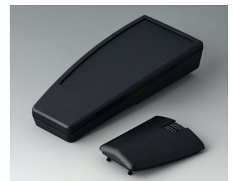
A9067209 SMART-CASE L, Vers. I PMMA (IR) (UL 94 HB) noir RAL 9005 140x62,7x30,5mm IP 40
