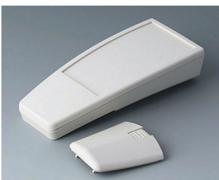
A9068107 SMART-CASE XL, Vers. I ABS (UL 94 HB) gris blanc RAL 9002 168x74,4x35,4mm IP 40
