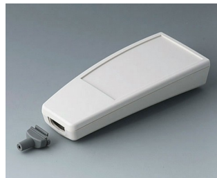
A9068137 SMART-CASE XL, Vers. IV ABS (UL 94 HB) gris blanc RAL 9002 168x74,4x35,4mm IP 65 opt., IP 40
