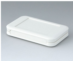
A9050107 SOFT-CASE S ABS (UL 94 HB) gris blanc RAL 9002 51x82x14mm IP 54 opt., IP 40
