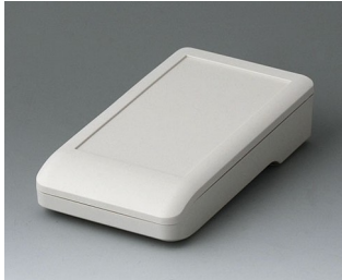
A9005107 DATEC-COMPACT S ASA+PC (UL 94 V-0) gris blanc RAL 9002 136x74x32mm IP 65
