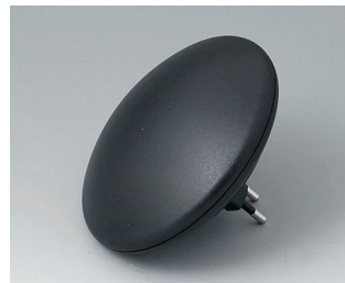
B5011129 ART-CASE R110 H PC+ABS (UL 94 V-0) noir RAL 9005 ø110x38mm IP 40
