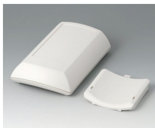
B7010107 ERGO-CASE M, plate ABS (UL 94 HB) gris blanc RAL 9002 150x100x40mm IP 54 opt.
