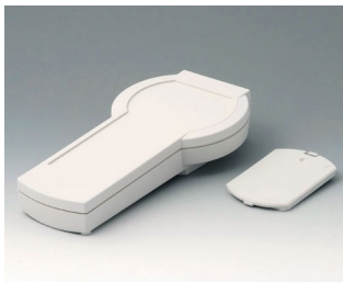
A9077107 DATEC-CONTROL S, Vers. I ABS (UL 94 HB) gris blanc RAL 9002 228x117x47mm IP 65 opt.
