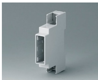
B6700100 RAILTEC C, 1 module, Vers. I PC (UL 94 V-0) gris clair 17,5x90x58mm
