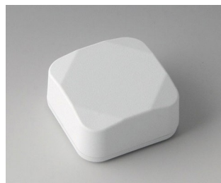
B1802217 MINI-DATA-BOX S40, haute ASA+PC (UL 94 V-0) blanc signalisation RAL 9016 40x40x20mm IP 65 opt., IP 40
