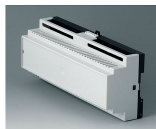
B6506118 RAILTEC B, 12 modules, Vers. IV PC (UL 94 V-0) gris clair RAL 7035 210x90x58mm
