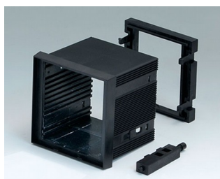
B6023011 BOITIER ENCASTRABLE TYPE A PPO (UL 94 V-0) noir RAL 9005 72x72x57mm
