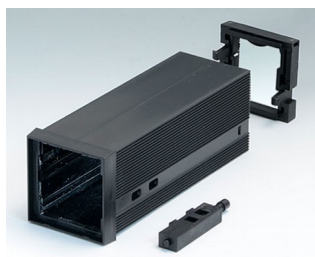
B6012061 BOITIER ENCASTRABLE TYPE A PPO (UL 94 V-0) noir RAL 9005 48x48x124mm
