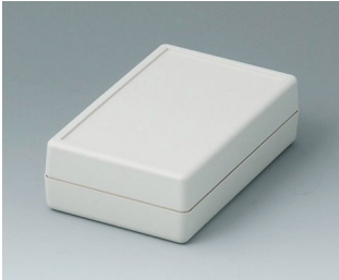
A9406351 BOITIER COQUILLES G 110, Vers. I ABS (UL 94 HB) gris blanc RAL 9002 72x114x33,5mm IP 65 opt.
