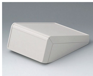
B4056117 UNITEC M, 1,4/1,4 ABS (UL 94 HB) gris blanc RAL 9002 148x210x80mm IP 40
