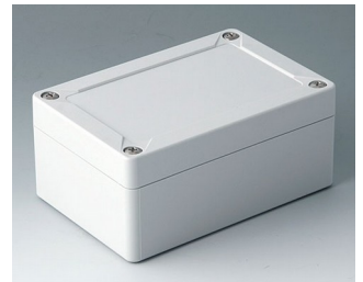
C7012011 IN-BOX ABS (UL 94 HB) lichtgrau RAL 7035 122x82x55mm IP 66, IP 67, IK 07
