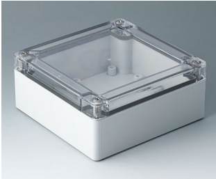
C7013034 IN-BOX ABS/PC (UL 94 HB) lichtgrau RAL 7035 124x122x55mm IP 66, IP 67, IK 07
