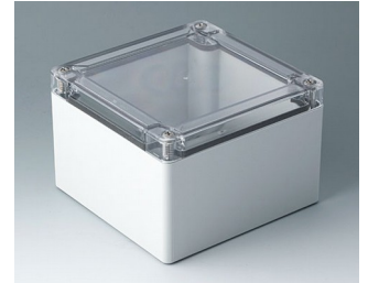
C7013054 IN-BOX ABS/PC (UL 94 HB) lichtgrau RAL 7035 124x122x85mm IP 66, IP 67, IK 07
