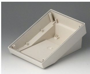
B4013117 DATEC-TERMINAL S ABS (UL 94 HB) grauweiß RAL 9002 130x180x86mm IP 54 opt.
