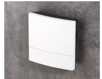
B3218201 NET-BOX 180, Ausf. II ASA+PC (UL 94 V-0) lichtgrau RAL 7035 180x180x48,5mm IP 65 opt.
