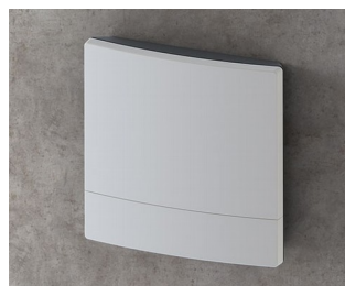
B3222201 NET-BOX 220, Ausf. II ASA+PC (UL 94 V-0) lichtgrau RAL 7035 220x220x50,5mm IP 65 opt.
