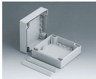
C2012122 ROBUST-BOX 120 BREIT, Ausf. II PC (UL 94 HB) lichtgrau RAL 7035 120x120x60mm IP 66
