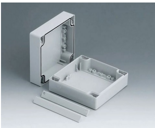
C2012121 ROBUST-BOX 120 BREIT, Ausf. I ABS (UL 94 HB) lichtgrau RAL 7035 120x120x60mm IP 66
