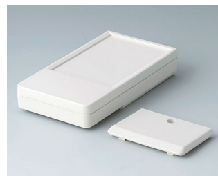
A9072117 DATEC-POCKET-BOX L ABS (UL 94 HB) grauweiß RAL 9002 120x65x22mm IP 54
