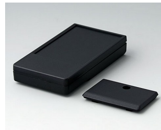
A9071209 DATEC-POCKET-BOX M PMMA (IR) (UL 94 HB) schwarz RAL 9005 105x58x18,5mm IP 41
