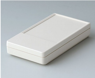
A9070107 DATEC-POCKET-BOX S ABS (UL 94 HB) grauweiß RAL 9002 85x46x16mm IP 41
