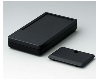
A9072209 DATEC-POCKET-BOX L PMMA (IR) (UL 94 HB) schwarz RAL 9005 120x65x22mm IP 41
