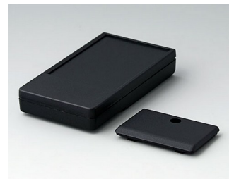
A9071219 DATEC-POCKET-BOX M PMMA (IR) (UL 94 HB) schwarz RAL 9005 105x58x18,5mm IP 54
