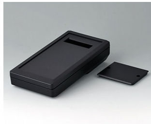
A9074209 DATEC-MOBIL-BOX M, Ausf. II ABS (UL 94 HB) schwarz RAL 9005 195x101x44mm IP 65 opt.
