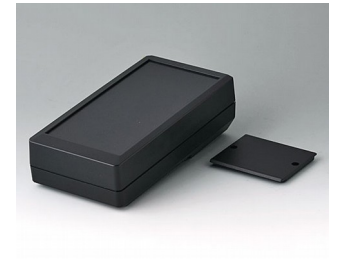
A9074129 DATEC-MOBIL-BOX M, Ausf. I, hoch ABS (UL 94 HB) schwarz RAL 9005 195x101x59mm IP 65 opt.
