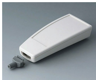
A9067147 SMART-CASE L, Ausf. V ABS (UL 94 HB) grauweiß RAL 9002 140x62,7x30,5mm IP 65 opt., IP 40
