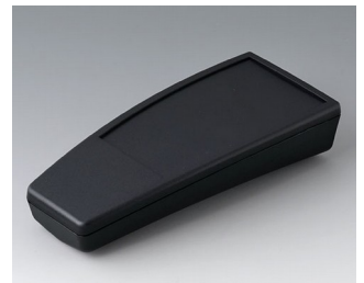
A9068219 SMART-CASE XL, Ausf. II PMMA (IR) (UL 94 HB) schwarz RAL 9005 168x74,4x35,4mm IP 65 opt., IP 40
