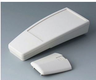
A9068107 SMART-CASE XL, Ausf. I ABS (UL 94 HB) grauweiß RAL 9002 168x74,4x35,4mm IP 40
