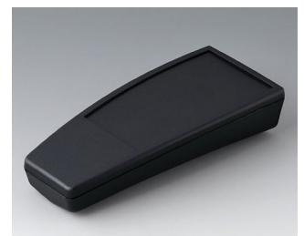
A9068119 SMART-CASE XL, Ausf. II ABS (UL 94 HB) schwarz RAL 9005 168x74,4x35,4mm IP 65 opt., IP 40
