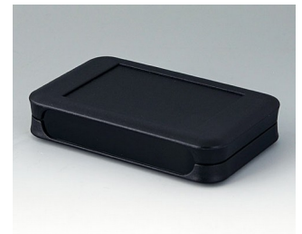
A9052209 SOFT-CASE L PMMA (IR) (UL 94 HB) schwarz RAL 9005 73x117x24mm IP 54 opt., IP 40
