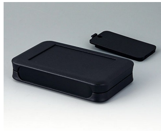
A9052229 SOFT-CASE L PMMA (IR) (UL 94 HB) schwarz RAL 9005 73x117x24mm IP 40
