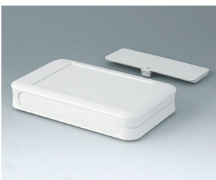
A9053117 SOFT-CASE XL ABS (UL 94 HB) grauweiß RAL 9002 92x150x28mm IP 40
