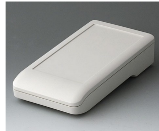
A9006117 DATEC-COMPACT M ASA+PC (UL 94 V-0) grauweiß RAL 9002 172x92x39mm IP 41
