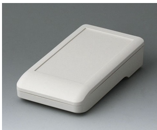
A9005107 DATEC-COMPACT S ASA+PC (UL 94 V-0) grauweiß RAL 9002 136x74x32mm IP 65
