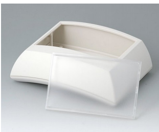
B7025147 ERGO-CASE L, hoch ABS (UL 94 HB) grauweiß RAL 9002 150x200x69mm IP 40
