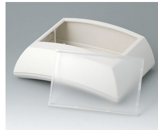
B7025247 ERGO-CASE L, hoch ABS (UL 94 HB) grauweiß RAL 9002 150x200x69mm IP 40
