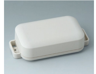
C3206207 EASYTEC 100 ASA+PC (UL 94 V-0) grauweiß RAL 9002 121x62x31mm IP 65 opt., IP 40
