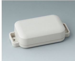
C3204207 EASYTEC 80 ASA+PC (UL 94 V-0) grauweiß RAL 9002 101x50x26mm IP 65 opt., IP 40
