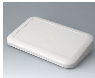
A9486107 EVOTEC 250, Ausf. III ASA+PC (UL 94 V-0) grauweiß RAL 9002 250x155x54mm IP 65 opt., IP 40
