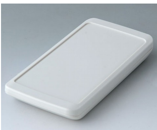
B5403307 SLIM-CASE M, Ausf. III ASA+PC (UL 94 V-0) grauweiß RAL 9002 148x74x19mm IP 65 opt., IP 40
