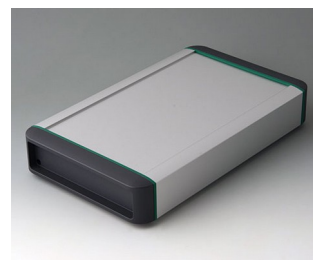
B3407031 SMART-TERMINAL 240 Aluminium AlMgSi 0,5 matt eloxiert 282x170x50mm IP 54
