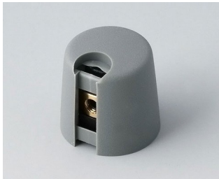
A1016048 TOP-KNOBS 16 PA 6 vulkan 16x16mm 4mm
