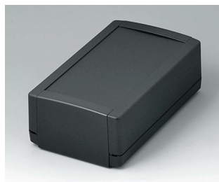
B1070369 TOPTEC 194 H, Ausf. I ABS (UL 94 HB) schwarz RAL 9005 194x115x68mm IP 40
