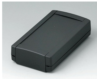
B1055369 TOPTEC 123 F, Ausf. I ABS (UL 94 HB) schwarz RAL 9005 123x68x30mm IP 40
